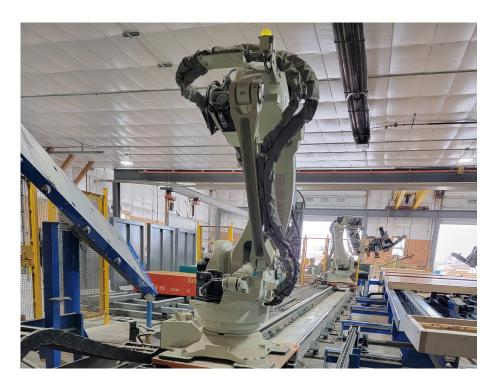
SCADAware created a one-of-a-kind system to automate much of this prefab assembly process using Güdel TrackMotion Technology.
