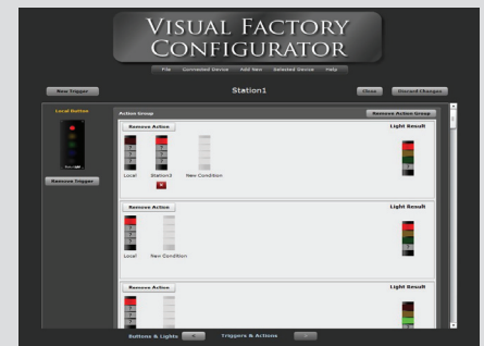
StatusLights can be configured to either flash or light steady based on button press sequences.
